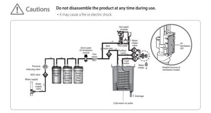
Consumables (Filter/Fitting/Tubing) should be genuine SK Magic products, and when replacing, ask a qualified technician for replacement. (It may cause a failure or the product life reduction.)
